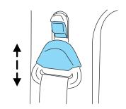
up. Pull down on the height adjuster to make sure it is locked in place.
